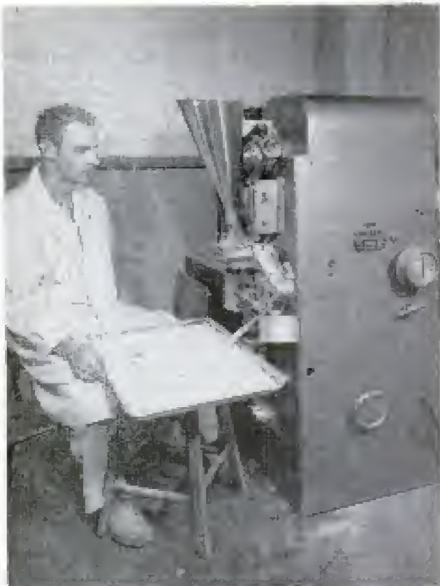
National Bureau of Standards photos Press stamps out ceramic wafers by the thousands, checks them for accuracy, rejects all faulty ones
